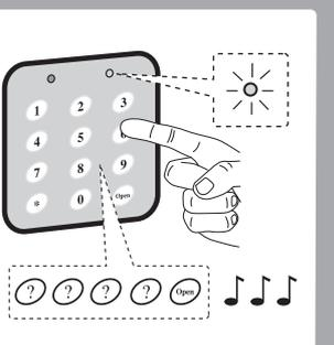
GB To check that your PIN code has been accepted operate the lock three times without closing the door. If unsure repeat the steps above.
